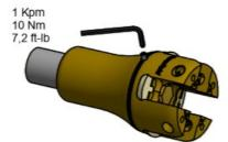
4 Align blade (6) with the blade socket in the hub and insert pivot pin (7) with the notch in pin aligned with the hole for the tapered pivot pin locking screw (8). Move blade slightly to ease operation. Correct if necessary using a screwdriver or similar tool.
