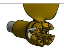
7 Mount sacrificial anode (11) Zn or AlMg, with the anode screw (12) pre-applied with threadlocker.
