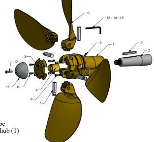
The cone on the shaft (2) must be degreased before mounting the hub (1)
