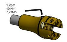
7 Mount sacrificial anode (11) Zn or AlMg, with the anode screw (12) pre-applied with thread locker.
