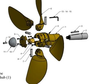
The cone on the shaft (2) must be degreased before mounting the hub (1)
