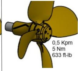
**3** Mount the shaft nut locking screw (5) using the supplied allen key. If using a torque wrench tighten twith 1 Kpm=10 Nm=7.2 ft-lb:
