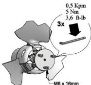
**6** Mount sacrificial anode (11) Zn or AlMg, with the anode screw (12). Finally, check the opening and folding
