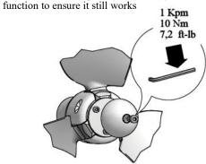
NOTE: If the anode screw has already been used, you have to apply new thread locker on the screw to reuse it.
