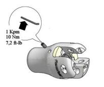
**3** Align blade (6) with the blade socket in the hub and insert pivot pin (7) with the notch in pin aligned with the hole for the tapered pivot pin locking screw (8). Move blade slightly to ease operation;
