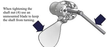
**2** Mount shaft nut locking screw (5) using the allen key (13) supplied. If using a torque wrench tighten twith 1 Kpm=10 Nm=7.2 ft-lb;
