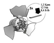
**5** Mount cover plate (9) with the three cover plate screws (10) using the allen key supplied; If using torque wrench tighten with 0.5 Kpm = 5 Nm = 3.6 ft-lb.
