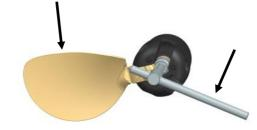
**2** Slide tab washer (5) onto the shaft nut locking screw (6).
