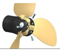
**8** Mount sacrificial anode (13) Zn or AlMg, with the anode screw (14). Move blades to check the opening and folding function to ensure it still works.
