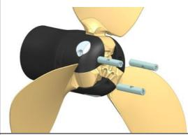
7 Mount cover plate (11) with the cover plate screws (12) using the allen key supplied. If using a torque wrench tighten with 5 Nm. Move blades to check the opening and folding function.
