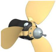
NOTE: If the anode screw has already been used, you have to apply new thread locker on the screw to reuse it.
