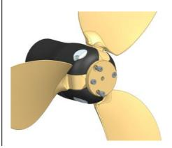
**8** Mount sacrificial anode (13) Zn or Al, with the anode screw (14). Tighten with 10 Nm. Move blades to check the opening and folding function to ensure it still works.
