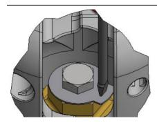
**2** Slide tab washer (5) onto the shaft nut locking screw (6).
