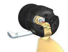
4 Align blade (7) with the blade socket in the hub and insert pivot pin (8) with the notch in pin aligned with the hole for the anchor pins (9).
