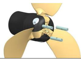
7 Mount cover plate (11) with the cover plate screws (12) using the allen key supplied. If using a torque wrench tighten with 5 Nm. Move blades to check the opening and folding function.
