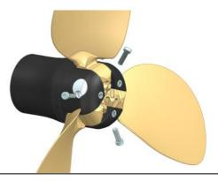
**8** Mount sacrificial anode (13) Zn or AlMg, with the anode screw (14). Tighten with 10 Nm. Move blades to check the opening and folding function to ensure it still works.
