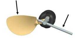
**2** Slide tab washer (5) onto the shaft nut locking screw (6).
