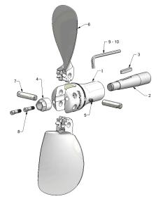
The cone on shaft (2) must be degreased before assembly of hub (1)
