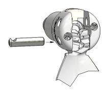
4 Insert one pivot pin locking screw (8); turn it to engage a couple of threads.
