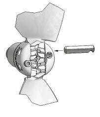
**6** Insert the last pivot pin locking screw (8); turn it to engage a couple of threads. It will be tightened later in step 7;
