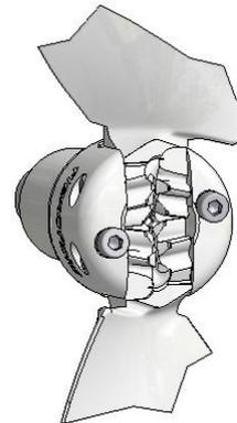
**5** Align the last blade (6) with the blade socket in the hub and insert pivot pin (7) with the notch in pin aligned with the hole for the pivot pin locking screw; Move blade slightly to ease operation.
