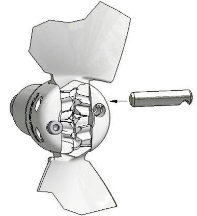
**7** Tighten both pivot pin locking screws (8) using the allen key (10) supplied; If using a torque wrench tighten with 1.2 Kpm=12 Nm=8.4 ft-lb;
