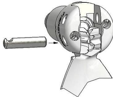
**4** Insert one pivot pin locking screw (8); turn it to engage a couple of threads. It will be tightened later in step 7.
