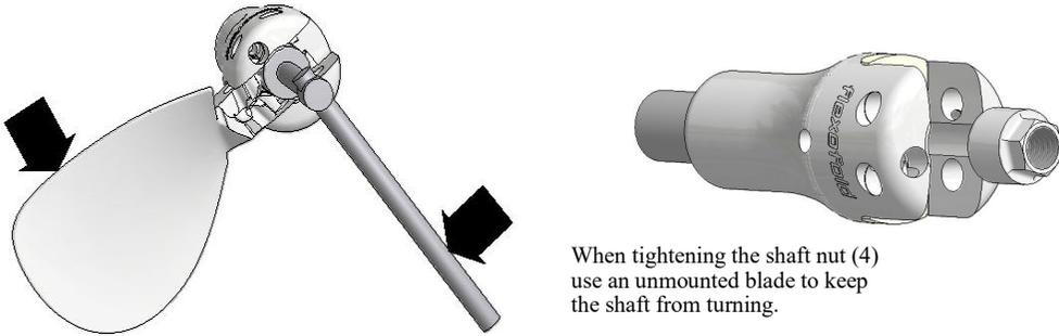
**2** Mount shaft nut locking screw (5) using the allen key (9) supplied. If using a torque wrench tighten with 1 Kpm=10 Nm=7.2 ft-lb;
