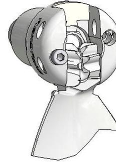
**6** Insert the last pivot pin locking screw (8); turn it to engage a couple of threads. It will be tightened later in step 7;
