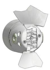
**8** Tighten both pivot pin locking screws (9) using the allen key (15) supplied; If using torque wrench tighten with 12 Nm:
