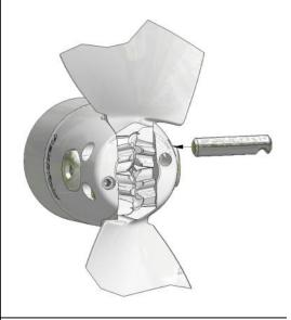
7 Insert the last pivot pin locking screw (9); turn it to engage a couple of threads; It will be tightened in step 8.
