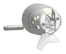
**5** Insert one pivot pin locking screw (9); turn it to engage a couple of threads; It will be tightened later in step 8.
