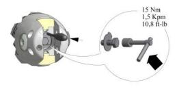
**3** Again using a straight screwdriver or similar; bend the opposite side of the tab washer up over one of the flat sides of the shaft nut locking screw (6)
