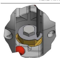
**2** Slide tab washer (5) onto the shaft nut locking screw (6). Attempt to position the tab relative to a flat side of the nut.
