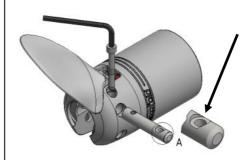
**4** Align blade (7) with the blade socket in the hub and insert pivot pin (8) with the stepped hole in the shown position.
