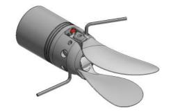
7 Release both anchor bolts approx. 1/8 turns counter clockwise (45 degrees). Check the function, i.e. work blades open and folded to ensure ease of operation.
